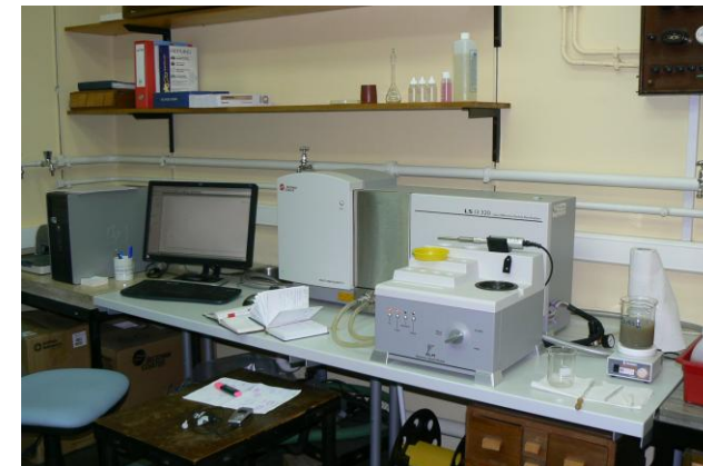
Grain size analyses (from the top left): wet sieving, sedigraph, laser granulometer
