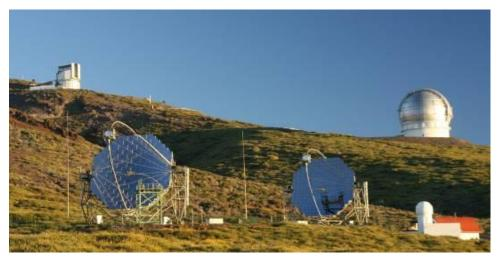
Photo of the two MAGIC telescopes on the Canary island of La Palma. The two 17m diameter telescopes measure the ultra-short flashes of bluish Cherenkov light, produced by the avalanches of secondary particles. These are produced by cosmic gamma rays that bombard the earth's atmosphere.
